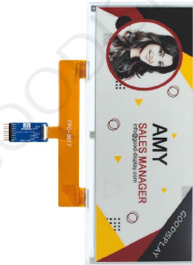
Figure 2 : Connection of E-paper display and Adapter
