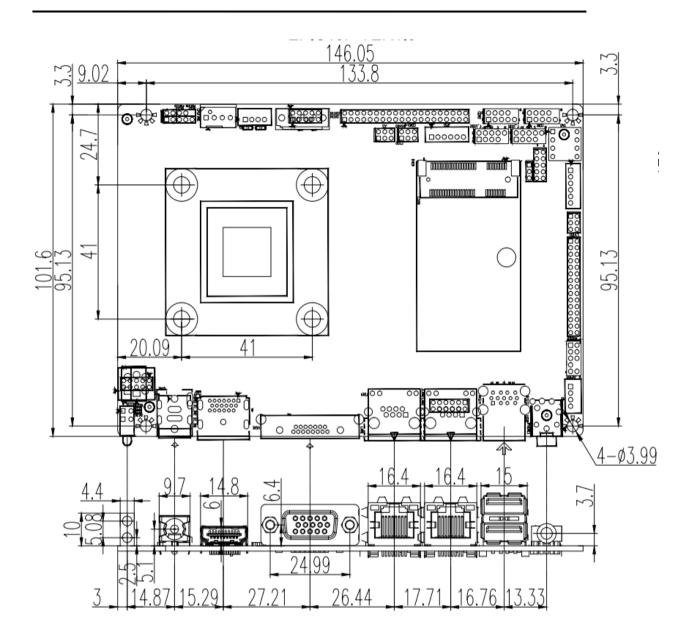
The above is the IO interface structure diagram of the EK-EPIC40P VER1.1 series motherboard
