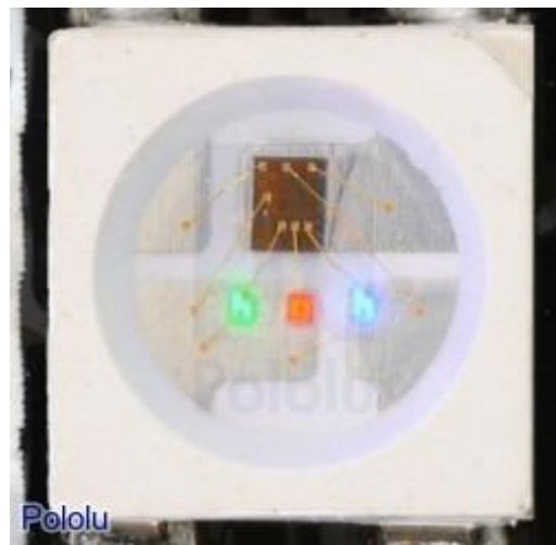
Close up of a WS2812B, with the red, green, and blue LEDs on at their dimmest setting.
