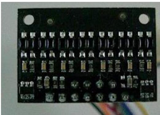
**Demo of IR LED dimming and independent even/odd control on the QTR-HD-07x (as seen through an old digital camera that can see IR).**
