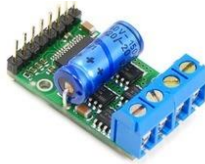
Pololu high-power motor driver with included components soldered in.
