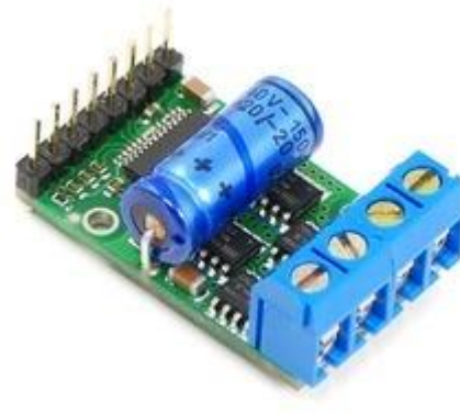
Pololu high-power motor driver with included components soldered in.
