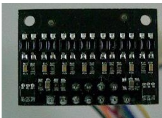
Demo of IR LED dimming and independent even/odd control on the QTR-HD-07x (as seen through an old digital camera that can see IR).
