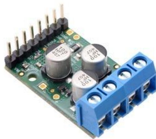
Pololu G2 High-Power Motor Driver 18v25 or 24v21 assembled with headers and terminal blocks.
