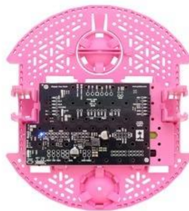
Motor Driver and Power Distribution Board for Romi Chassis mounted on a chassis prior to motor installation.
