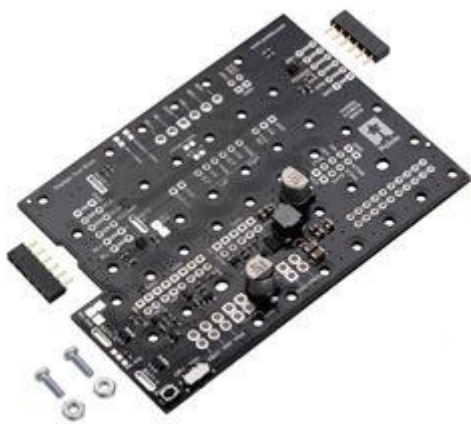
Motor Driver and Power Distribution Board for Romi Chassis with included hardware.
