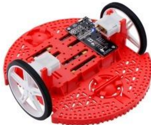
Power Distribution Board for Romi Chassis.
