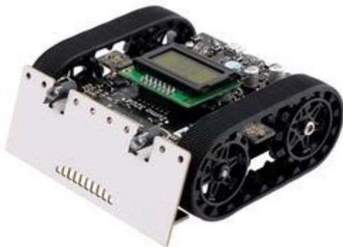
Assembled Zumo 32U4 robot.
