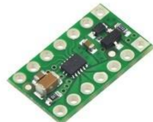
DRV8835 dual motor driver carrier.
