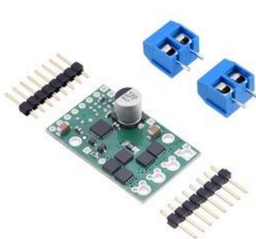
Pololu G2 High-Power Motor Driver 18v17 or 24v13 with included hardware.
