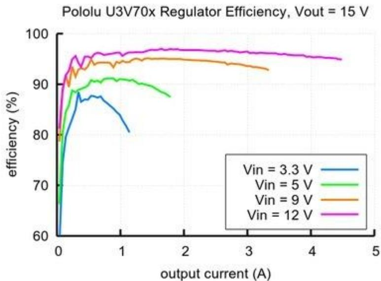
The maximum achievable output current is approximately proportional to the ratio of the input voltage to the output voltage. Additionally, the maximum output current can depend on other factors, including the ambient temperature, air flow, and heat sinking. The graph below shows the typical maximum continuous output currents these regulators can deliver at room temperature with no forced airflow or heat sinking.
