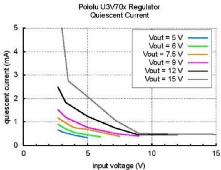
Typical maximum quiescent current of Step-Up Voltage Regulator U3V70x (regulator enabled, no load).
