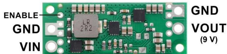
The input voltage, **VIN**, must be at least 2.9 V and should not exceed the output voltage, **VOUT**. (If **VIN** is higher than **VOUT**, the higher input voltage will show up on the output, which is potentially dangerous for your connected load and could also damage the regulator.)
