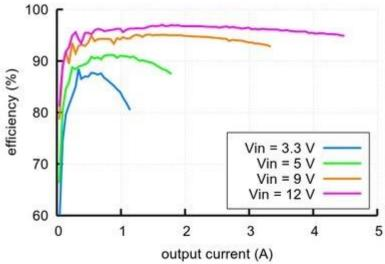
The maximum achievable output current is approximately proportional to the ratio of the input voltage to the output voltage. Additionally, the maximum output current can depend on other factors, including the ambient temperature, air flow, and heat sinking. The graph below shows the typical maximum continuous output currents these regulators can deliver at room temperature with no forced airflow or heat sinking.
