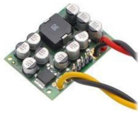
Pololu Step-Down Voltage Regulator D24V150Fx showing wires soldered directly to the board.
