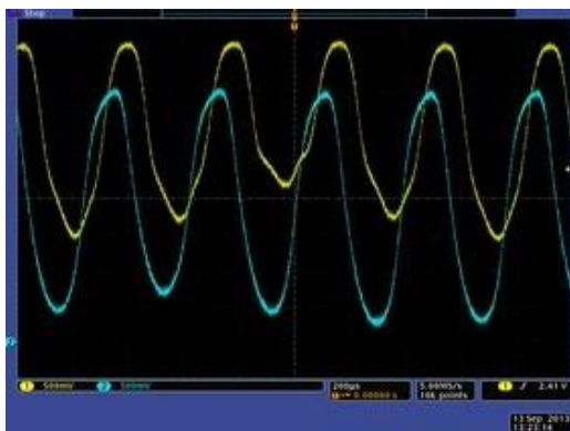
5V encoder version, motor approx. 30k RPM: 5-tooth wheel slightly too close to sensors.
