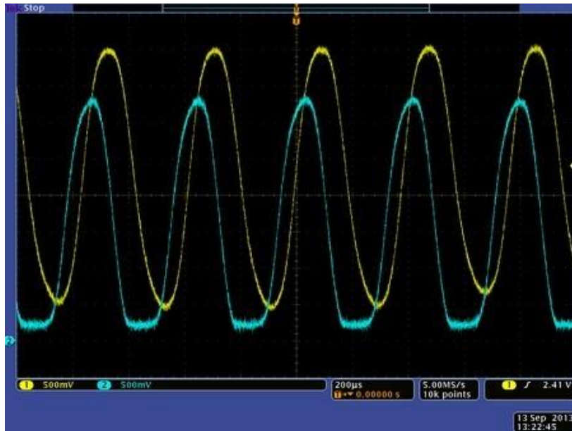
5V encoder version, motor approx. 30k RPM: 5-tooth wheel at optimal distance from sensors.
