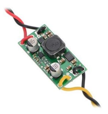
The board has four 0.086" mounting holes intended for #2 or M2 screws. In applications where mounting screws are not used and wires are soldered directly to the board, the insulated part of the wires can be passed through the mounting holes for strain relief. The picture above shows an example of this with 20 AWG wire, which was close to the limit of what would fit through the mounting holes.
