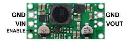
The input voltage, VIN, should be between 2.9 V and 32 V. Lower input voltages can cause the regulator to shut down or behave erratically; higher input voltages can destroy the regulator, so you should ensure that noise on the input is not excessive. 32 V should be treated as the absolute maximum input voltage. Our recommended maximum operating voltage is 30 V, which is the limit of the reverse voltage protection.
