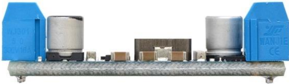
Pololu step-up voltage regulator U3V50x with included terminal blocks installed, side view.
