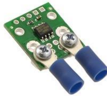
ACS711 current sensor carrier (LC package version) with solderless ring terminal connectors (not included).
