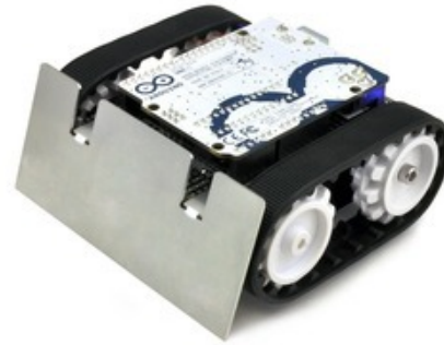
Assembled Zumo robot for Arduino with an Arduino Uno (with original white sprockets).
