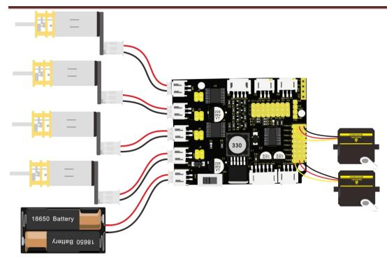
Note: PWM8-PWM15 is only connected to 2 servos on above diagram, in the code , PWM8-PWM15 controls 8 servos to test.
