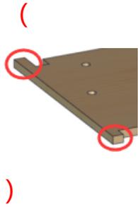
Install the protruding ends of board A gently because they are weak
