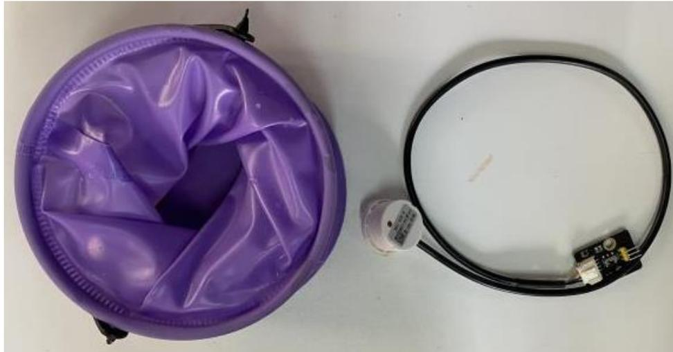
Mount the non-contact liquid level sensor onto flexible barrel
