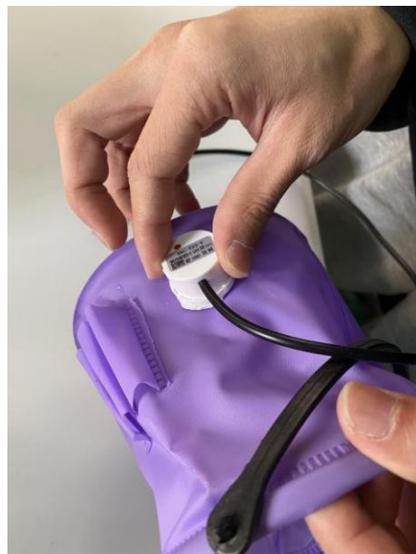
Glue the sensor onto barrel after tearing off the thin film
