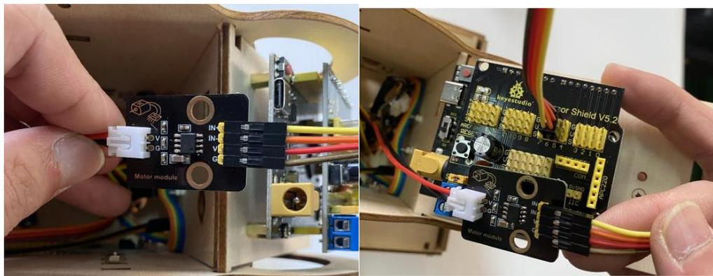
Attach the end of water pump to motor driver module, then
