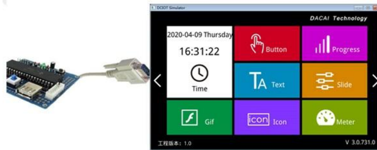
Diagram 12-2 Onlinedebugging of serial port of user's single-chip microcomputer and virtual serial port screen
