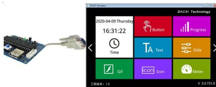
Diagram 11-2 Online debugging of serial port of user's single-chip microcomputer and virtual serial port screen
