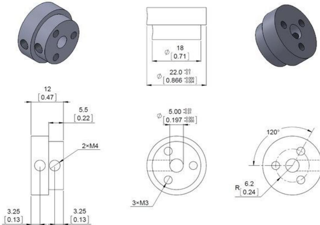
Dimension diagram of the Pololu aluminum scooter wheel adapter threaded mount for 5 mm shafts. Units are mm over [inches].
