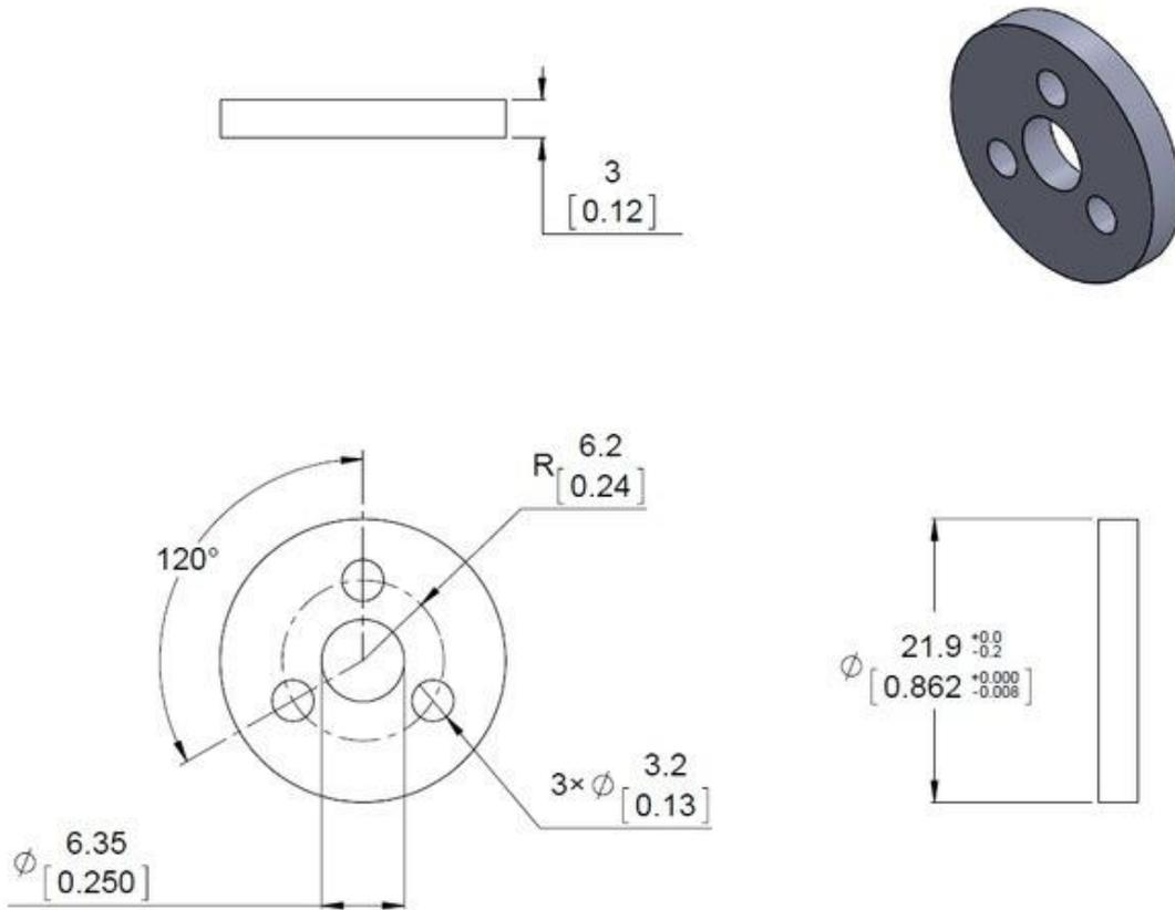
Dimension diagram of the Pololu aluminum scooter wheel adapter flat washer.
