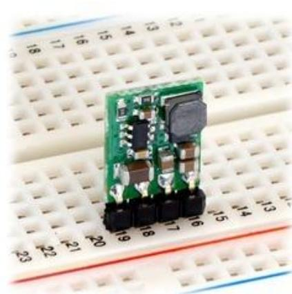
The SHDN pin can be driven low (under 0.3 V) to turn off the output and put the board into a low-power state that typically draws 20  $\mu$ A, and it can be driven high (above 2.3 V) to enable the board. If you do not need to use the shutdown feature, the SHDN
