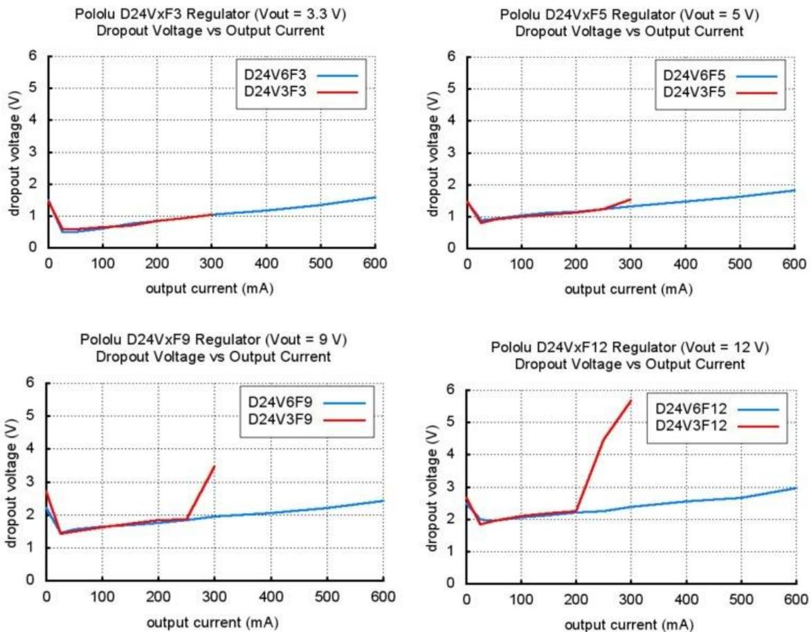
As you can see from the last two graphs, the dropout voltage of the low-current 9 V and 12 V versions (D24V3F9 and D24V3F12) spikes as the output current nears the 300 mA limit. For similar regulators with much lower dropout voltages, please consider our newer 500 mA [D24V5Fx buck regulators](https://eckstein-shop.de/).
