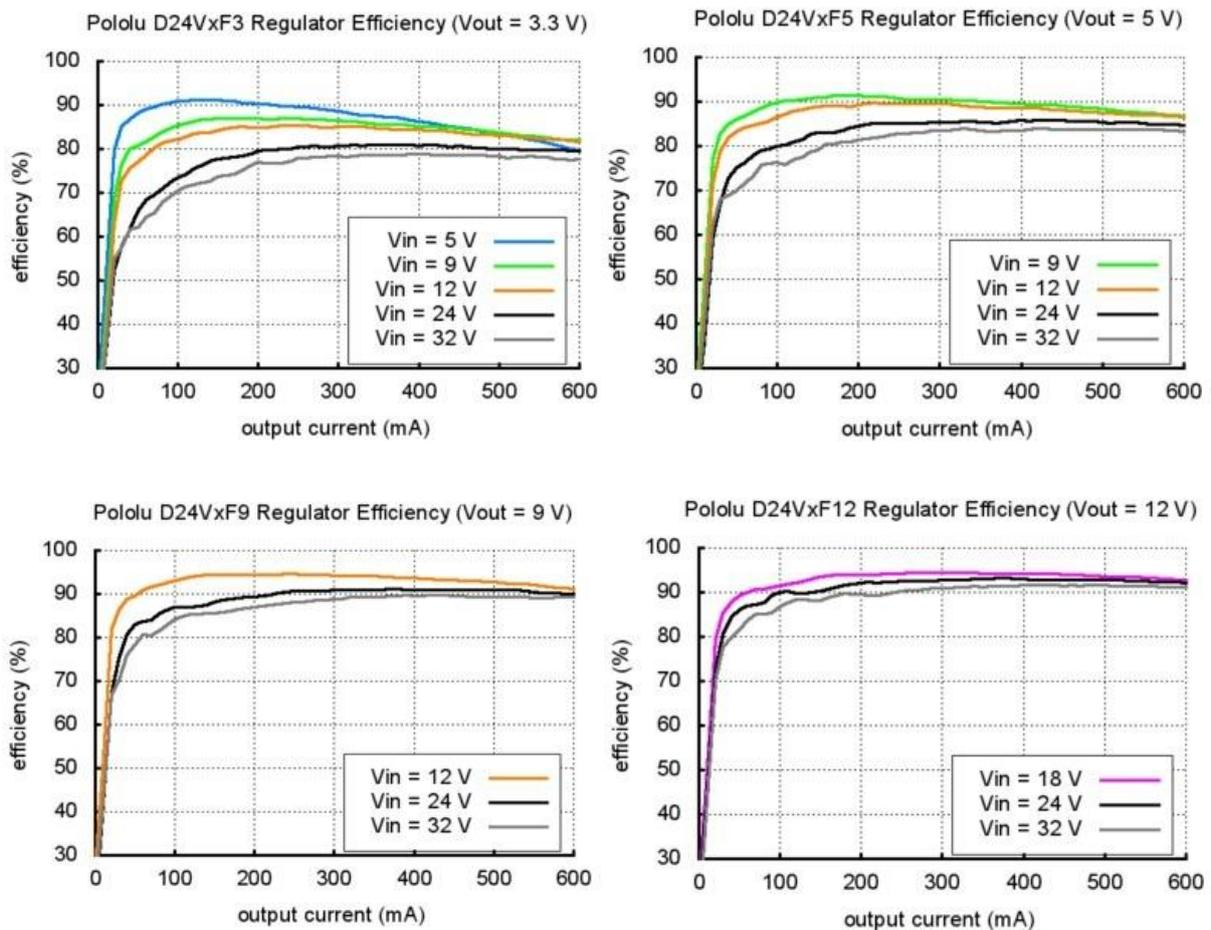
Note that the above graphs apply to both the 300 mA and 600 mA versions, which is why the x axis extends to 600 mA. You should not expect to get more than 300 mA from the 300 mA versions (D24V3Fx). These graphs and ones below do not apply to our newer 500 mA [D24V5Fx buck regulators](#), which have different operating characteristics, including much lower dropout voltages.
