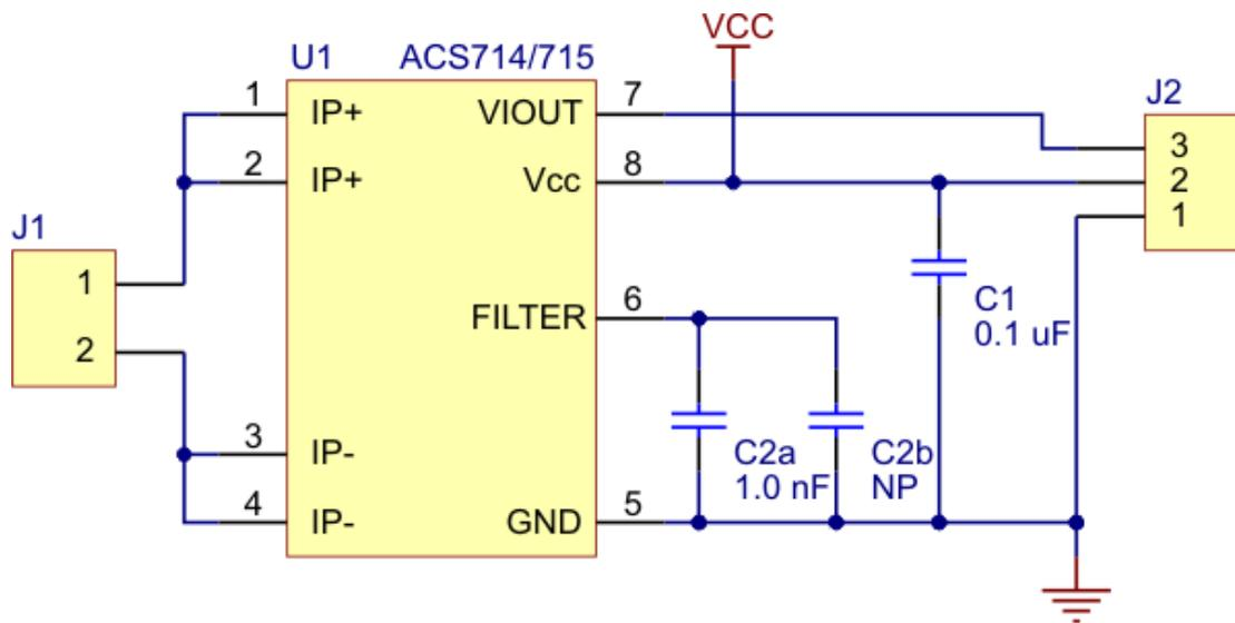
Pololu ACS714/ACS715 current sensor carrier schematic diagram.
